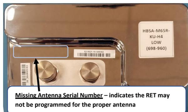
**Any RET not labeled with the antenna serial number must be assumed to be a raw bulk spare and the same warnings noted above will apply.**
